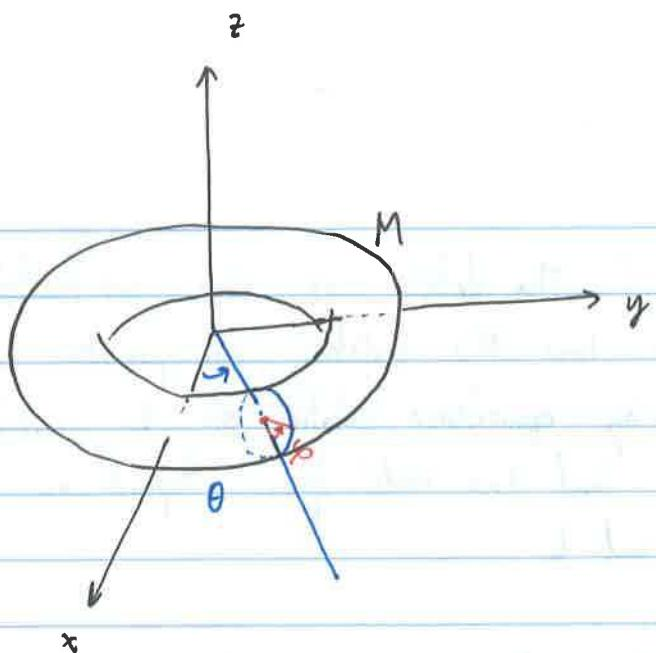
$$\begin{aligned}x &= (a + b \cos \varphi) \cos \theta \\y &= (a + b \cos \varphi) \sin \theta \\z &= b \sin \varphi\end{aligned}$$
