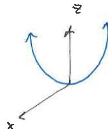
Since  $y$  can be any real number (it's not in equation), then this forms a parabolic cylinder.
