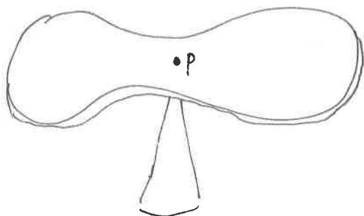
$P$  = the center of mass <sup>(gravity)</sup>
