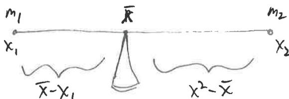
Two masses are attached to opposite ends of a rod. We do we need to put the fulcrum so that the rod will balance?
