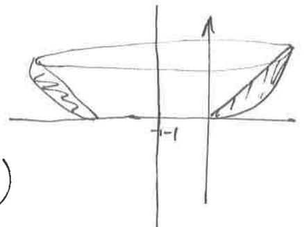
$$V = \pi \int_0^1 -y^2 - y + 2y^{1/2} dy = \pi \left( -\frac{1}{3}y^3 - \frac{1}{2}y^2 + \frac{4}{3}y^{3/2} \right) \Big|_0^1 = \pi \left( \frac{4}{3} - \frac{1}{2} - \frac{1}{3} \right) = \boxed{\frac{\pi}{2}}$$
