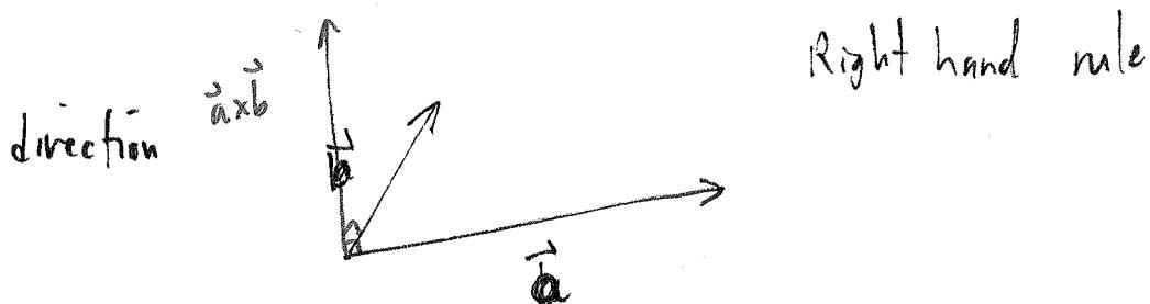
(2) length:  $|\vec{a} \times \vec{b}| = \text{area of parallelogram}$
