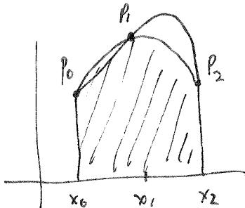
Uses a parabola that passes thru  $P_0$ ,  $P_1$ , and  $P_2$ .
