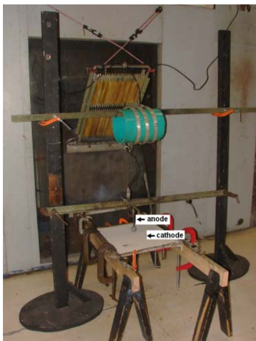
FIG. 1 HIGH-CURRENT, DIRECT EFFECTS LABORATORY LIGHTNING TESTING: SCHEMATIC OF THE STANDARDIZED SIMULATED LIGHTNING WAVEFORM WITH CURRENT COMPONENTS AND A PHOTOGRAPH OF THE TEST SETUP AT LIGHTNING TECHNOLOGIES, INC.
