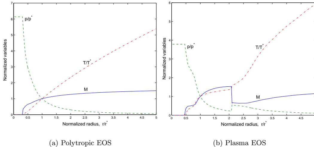
**Figure 3.** Normalized ablated gas profiles at  $10 \mu s$  in 1D spherically symmetric model of (a) ablation without atomic processes (polytypic EOS), and (b) with atomic processes (plasma EOS). The solid, dashed, and dash-dotted lines are  $M$ ,  $p/p^*$ , and  $T/T^*$  as functions of  $r/r^*$ , respectively.
