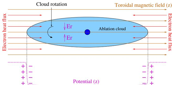
**Figure 1.** Schematic of physics processes associated with the ablation of deuterium pellet in a tokamak.
