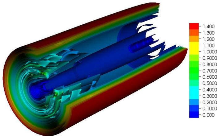
**Figure 5.** Isosurfaces of rotational Mach number in the steady-state ablation cloud.
