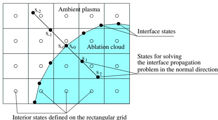
**Figure 2.** Rectangular grid, interface, and states for the method of front tracking. States contain density, momentum, and energy density of the fluid (plasma) and references to the EOS model and other parameters.
